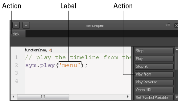
Figure 20-3: Add a Click, Play From action to create a link to the sub-level menu.
