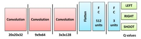
Figure 3-7. Example Architecture for Deep Q Network
