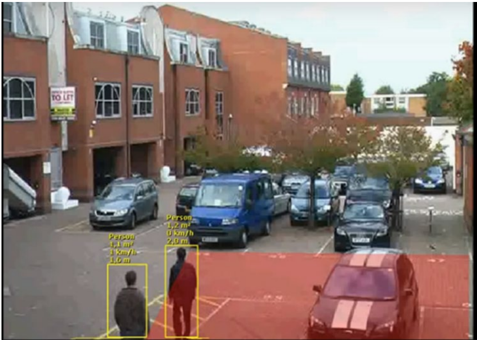
Figure 8-15. Object-detecting video surveillance system
