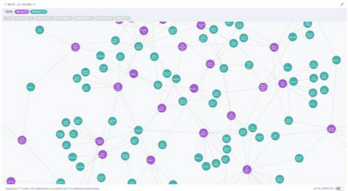
Figure 2-3. The graph view of running a MATCH (n) RETURN n; query on the Neo4j movie database
