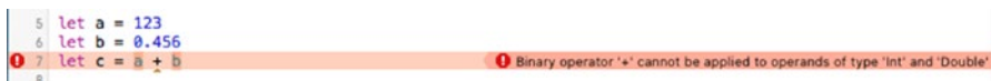
Figure A-5. Swift does not allow you to combine variables of different types
