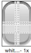
Figure 4-27. This is what the default slicing for the white button looks like
