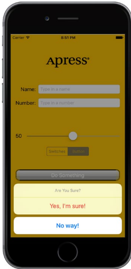
Figure 4-3. Our application uses an action sheet to elicit a response from the user
