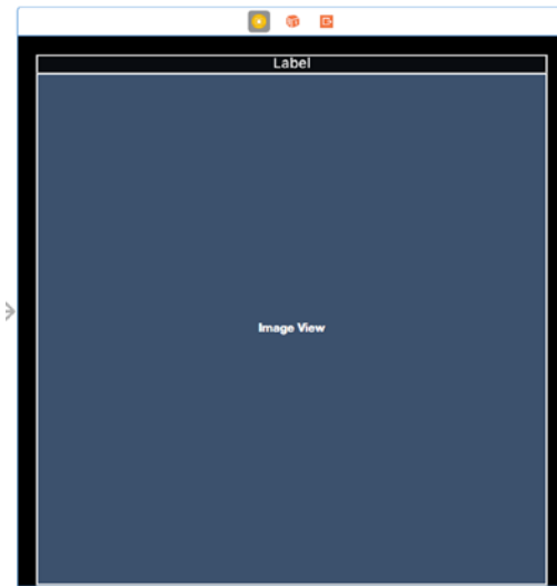
Figure 10-9. The vertical stack view with its nested views as they will be at run time
