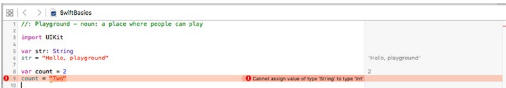
Figure A-3. Swift is not a dynamic language. You can't change the type of a variable
