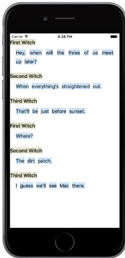
Figure 10-1. Each word is a separate cell, with the exception of the headers, which are, well, headers. All of this is laid out using a single UICollectionView , and no explicit geometry calculations of our own
