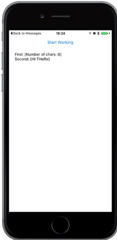
Figure 15-1. The SlowWorker application hides its interface behind a single button. Click the button, and the interface hangs for about ten seconds while the application does its work
