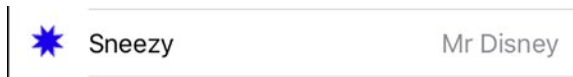
Figure 8-10. The style value 1 places the text label on the left side in black letters and the detail text right-justified on the right side in blue letters
