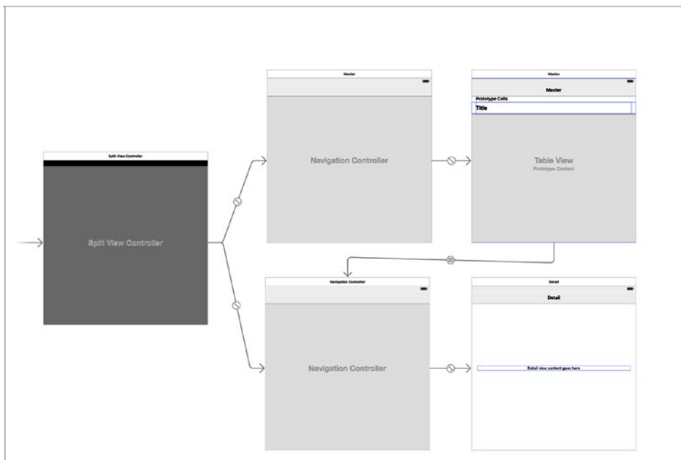
Figure 14-2. The TinyPix storyboard, showing split view controller, navigation controllers, master view controller, and detail view controller
