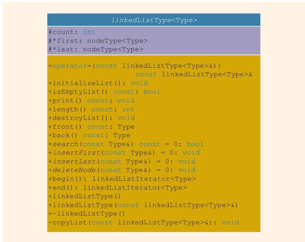
FIGURE 17-20 UML class diagram of the class linkedListType
