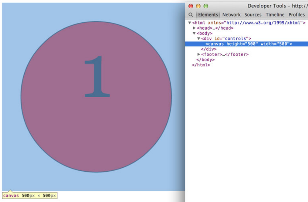
Figure 8.7 Any graphics created in canvas are stored as a bitmap or raster image. Unlike in SVG, the individual shapes are no longer accessible or modifiable after being drawn.
