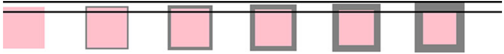
Figure 1.19 The same 25 x 25 <rect> with no, 1-px, 2-px, 3-px, 4-px, and 5-px strokes. Though these are drawn on a retina screen using half-pixels, the second and third report the same width and height (27 px x 27 px) as the fourth and fifth (29 px x 29 px).
