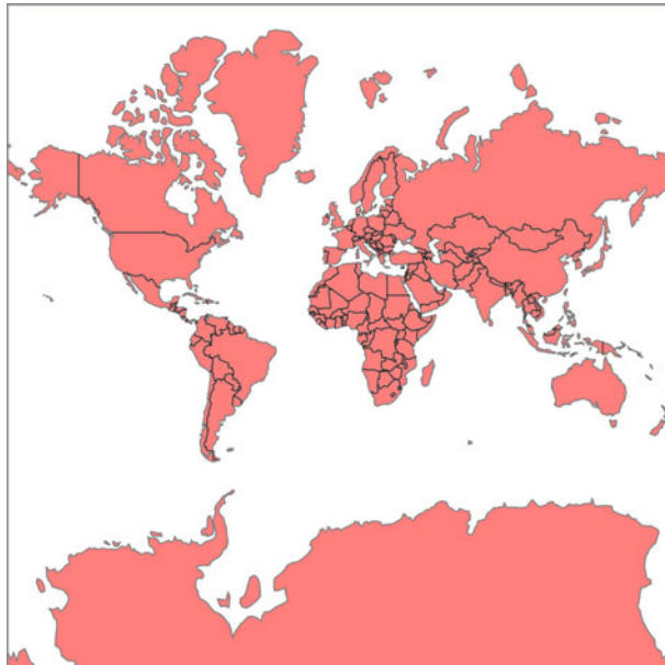
Figure 7.4 The Mercator-projected world from our data now fitting our SVG area. Notice the enormous distortion in size of regions near the poles, such as Greenland and Antarctica.
