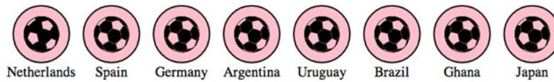
Figure 3.23 Each <g> element has its own set of paths cloned as child nodes, resulting in football icons overlaid on each element.
