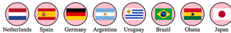
Figure 3.18 Our graphical representations of each team now include a small PNG national flag, downloaded from Wikipedia and loaded using an SVG <image> element. 🇳🇱
