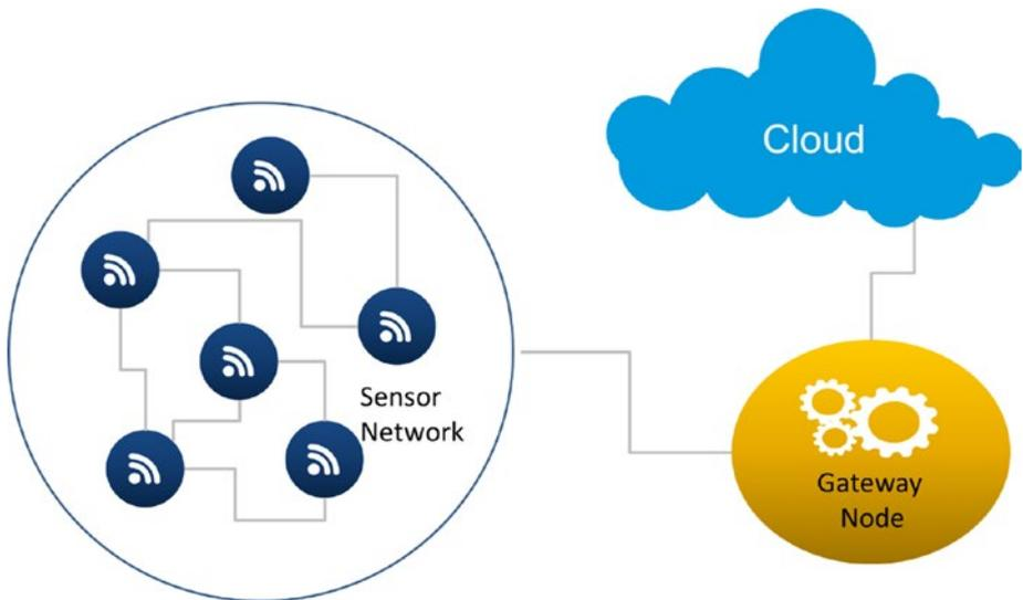
*Figure 1-4. Device-to-gateway framework*
