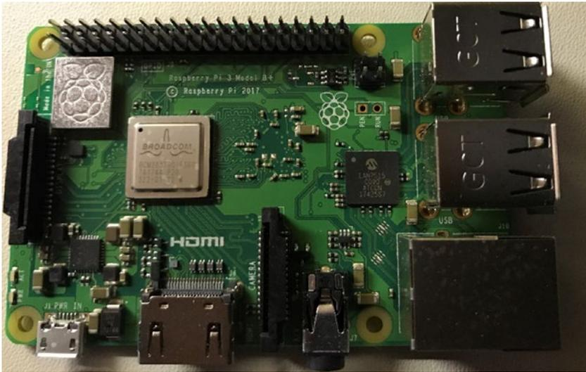
**Figure 6-1.** *Raspberry Pi 3 Model B+*
