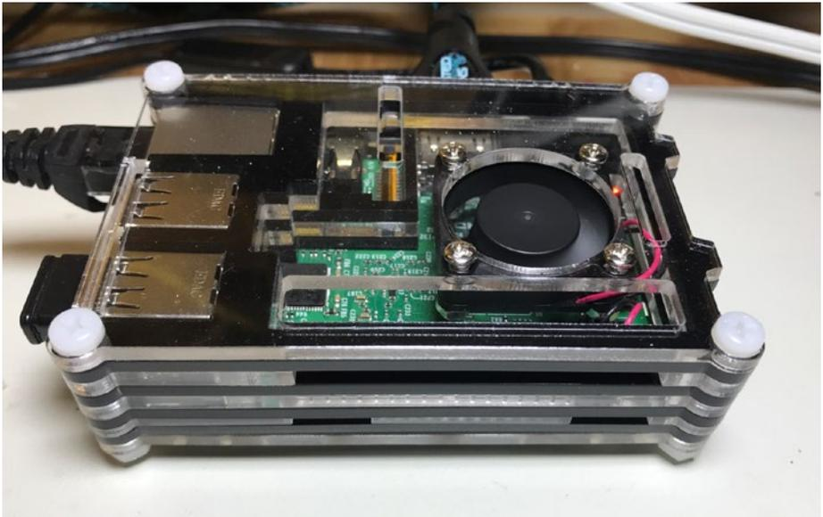
**Figure 6-2.** *Raspberry Pi in ruggedized Smraza case*
