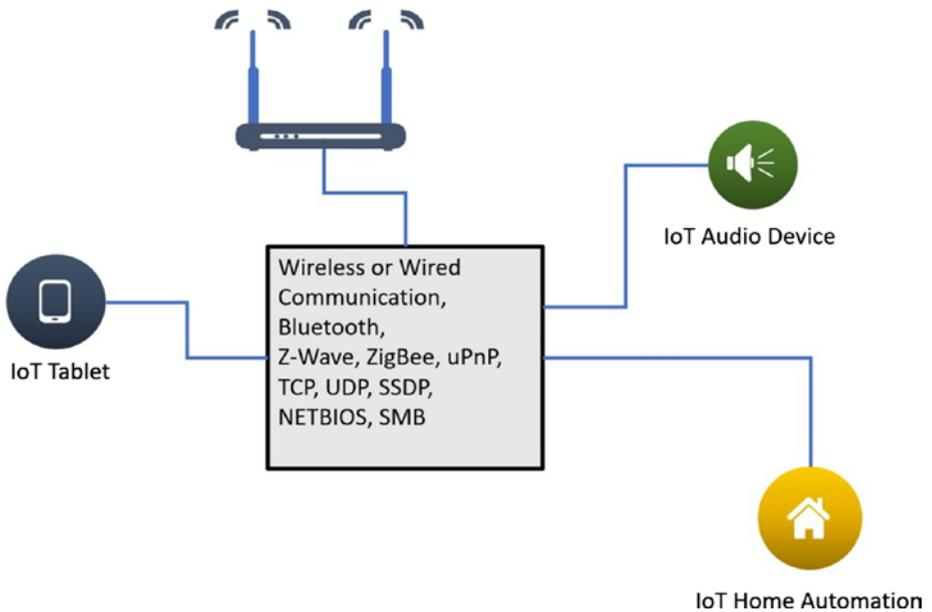
**Figure 1-2.** *Device-to-device communication model*
