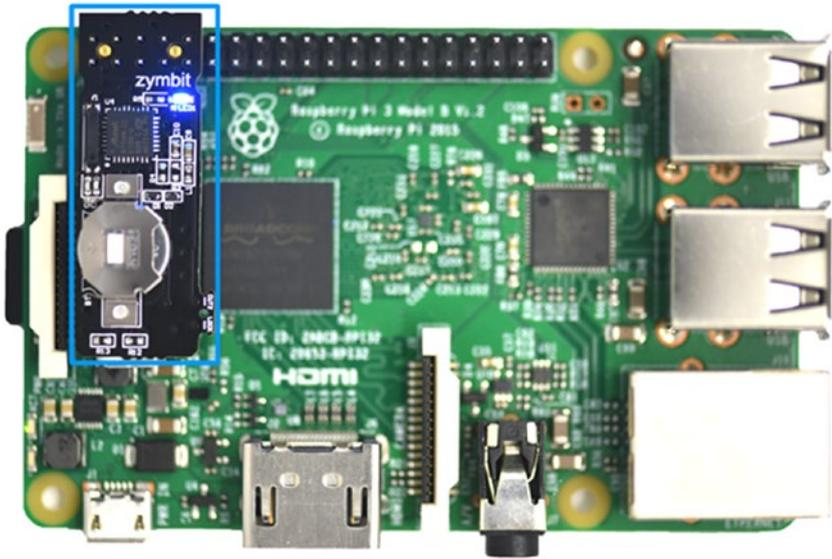
**Figure 7-2.** ZYMKEY install on a Raspberry Pi
