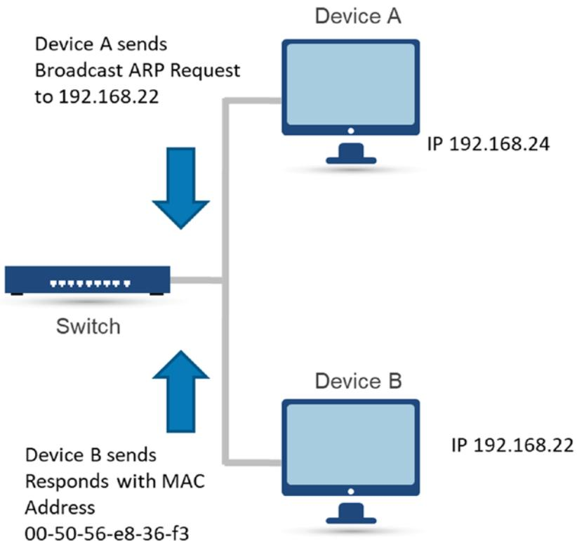
**Figure 2-4.** Simplified ARP request/replay process
