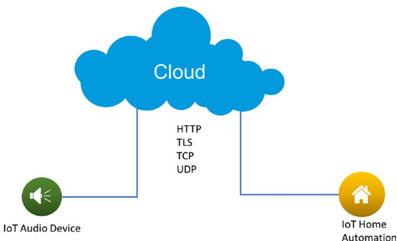
*Figure 1-3. Device-to-cloud communication*
