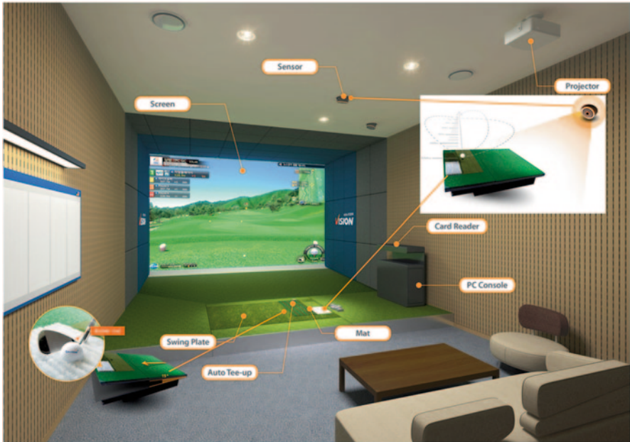
Fig. 5.3 An interaction case that uses metaphors: virtual golf simulator (courtesy of GolfZon, used with permission)
