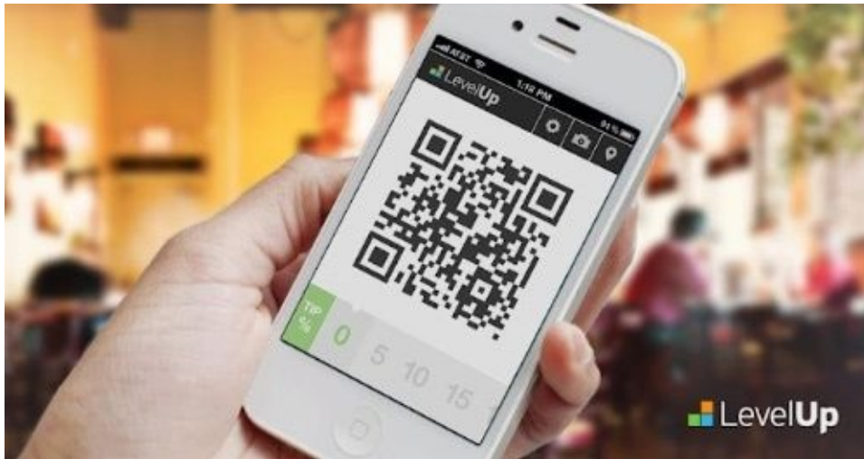
Figure 2-8. LevelUp uses QR codes, which are linked to a credit or debit card stored in the cloud (image courtesy of LevelUp)
