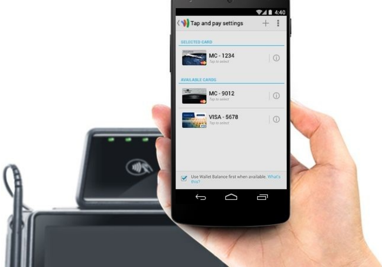
Figure 2-1. Google Wallet is one example of NFC payments in the United States: once users link their cards to their Wallet account, they can tap their phone at any NFC-enabled point of sale (image courtesy of Google)
