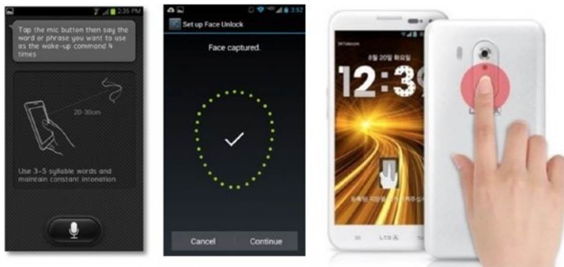
Figure 7-16. Examples of unlocking a device with voice commands, facial recognition, and fingerprint scans
