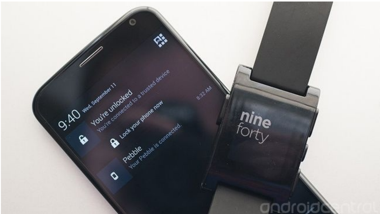
Figure 4-28. The Pebble watch added as a trusted device to Moto X, which enables unlocking the phone as long as the two devices are in Bluetooth connection proximity (source: AndroidCentral [48] )
