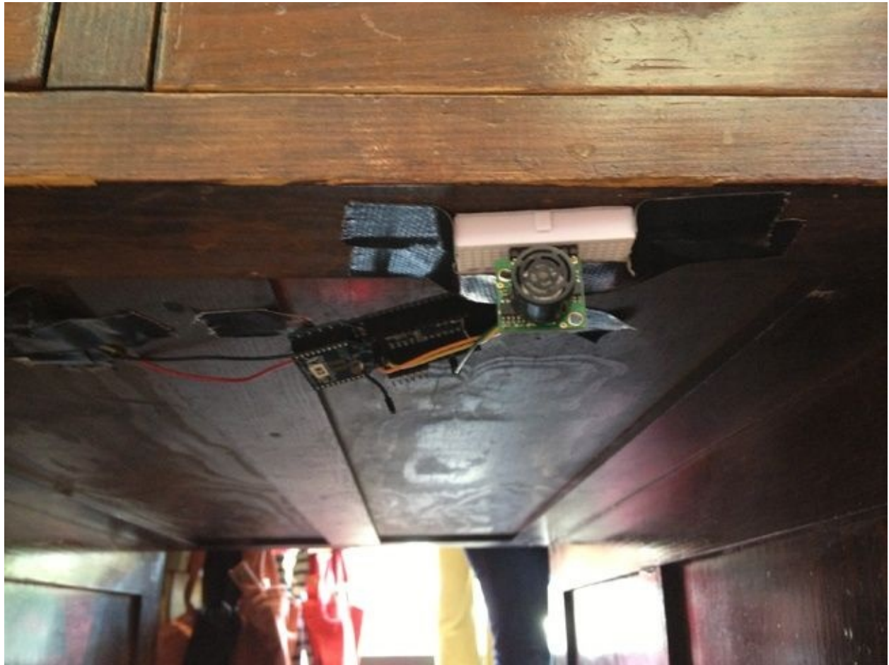
Figure 9-5. A bare sensor taped under a display table in Tigertree
