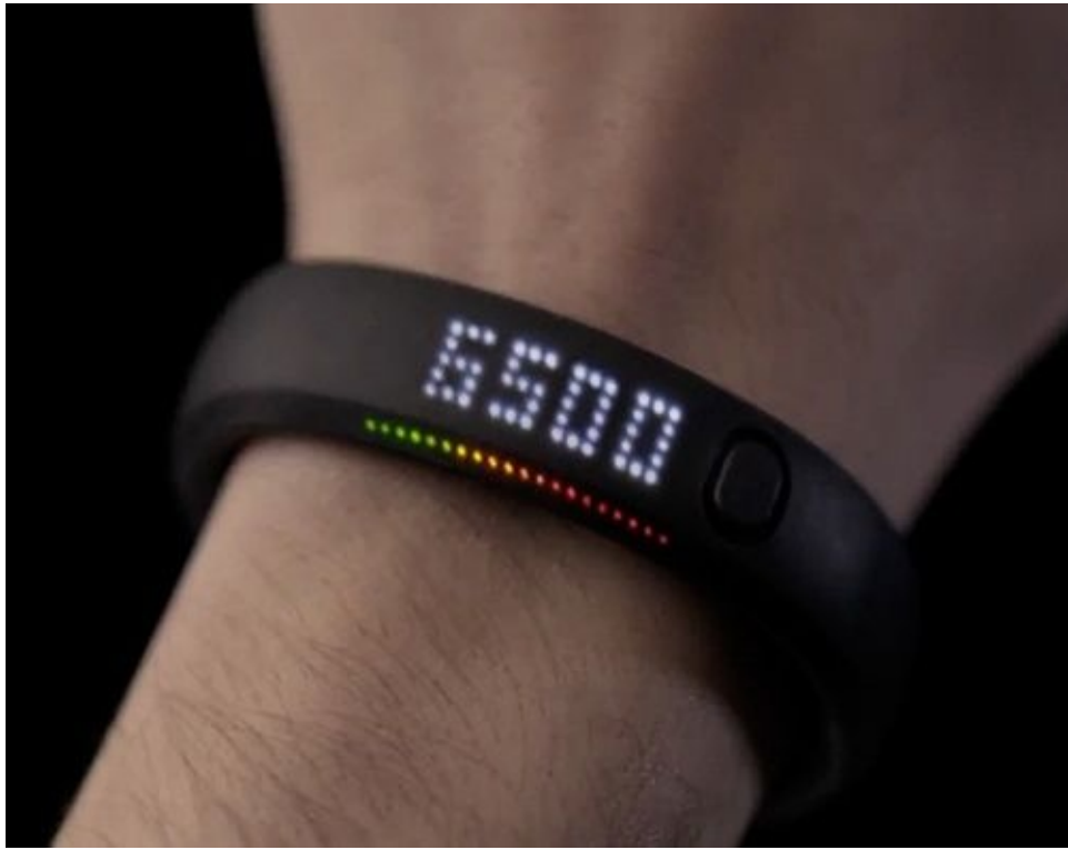
Figure 4-23. The Nike+ FuelBand provides both exact numbers (such as numbers of steps) along with a visual indication about the progress in relation to the daily goal
