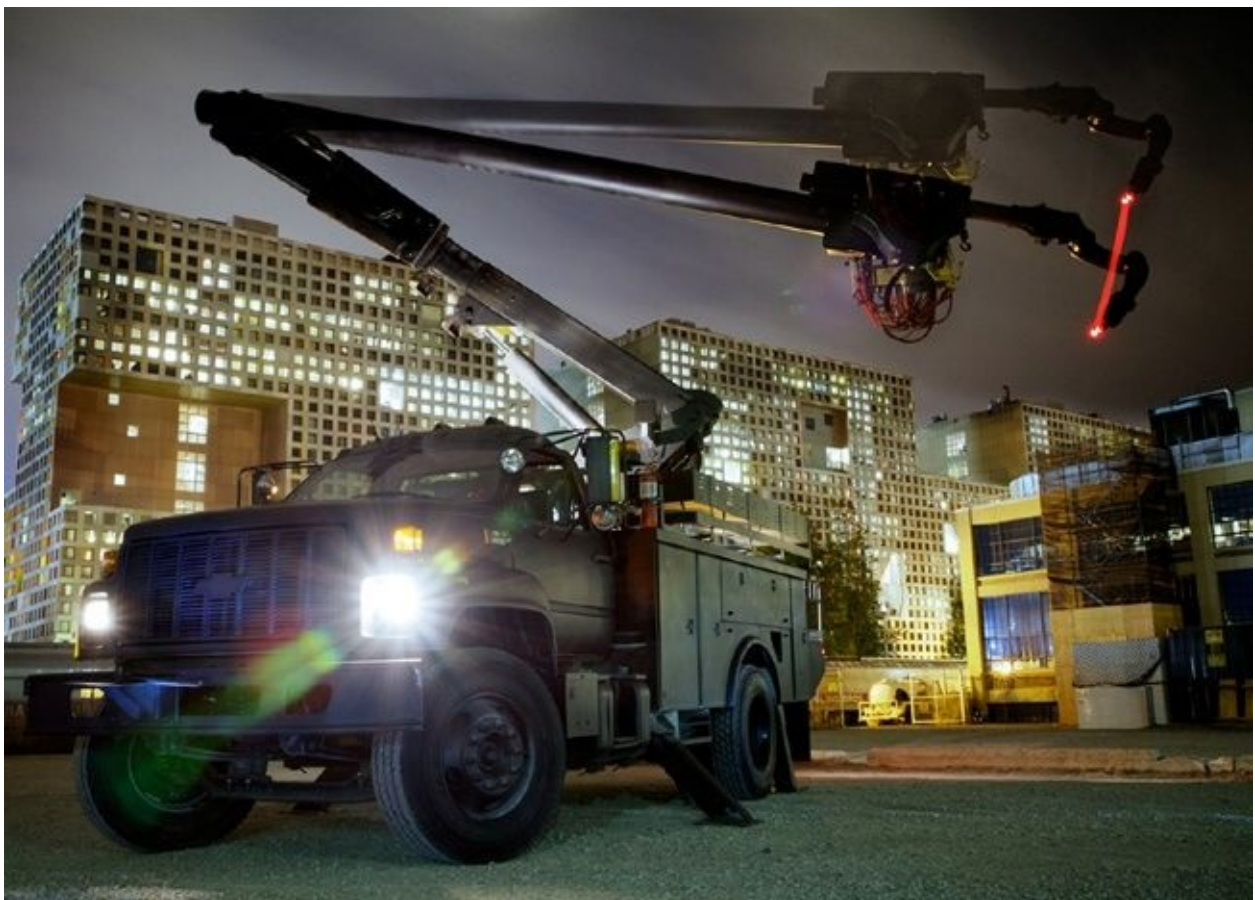
Figure 18-1. The Digital Construction Platform comprises a six-axis KUKA robotic arm mounted to a five-axis Altec hydraulic boom arm
