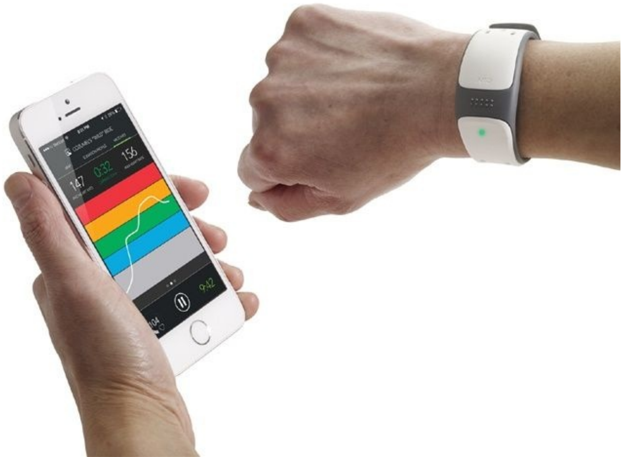
Figure 4-19. Mio LINK, which uses a single on-device LED to provide feedback about the heart rate state
