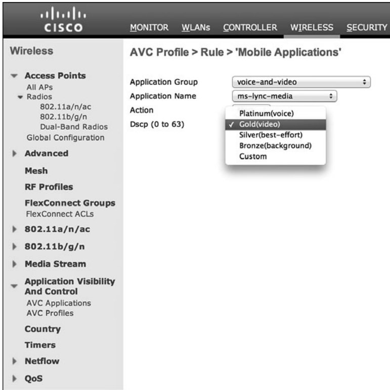
Figure 19-13 Re-marking DSCP Using AVC
