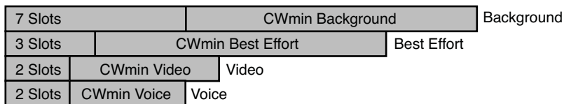
Figure 18-5 AIFS and Contention Window Sizing
