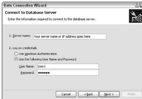
Figure 12-7: Step 1 of the Data Connection Wizard is to enter some authenti- cation information.
