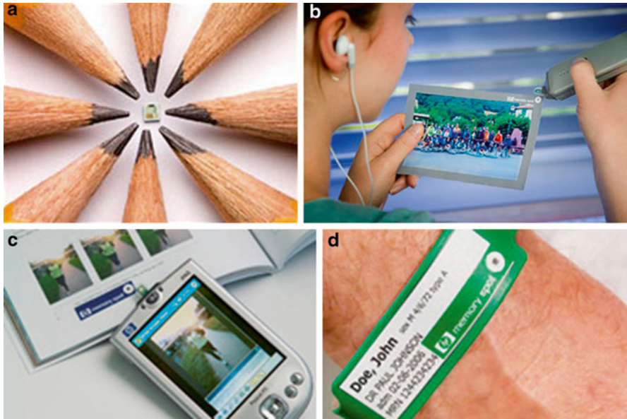
Fig. 7.4 HP memory spot (a) and its potential applications, (b) a printed audiophoto, (c) a talking book, and (d) a hospital wristband (Reprinted with permission)
