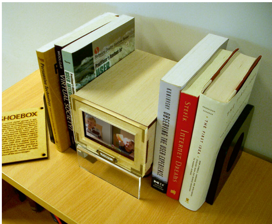
Fig. 8.10 The shoebox prototype (Banks and Sellen 2009). The top of the box lifts up to reveal a stack of pseudo-transparency cases for touch-based selection (Used with permission)
