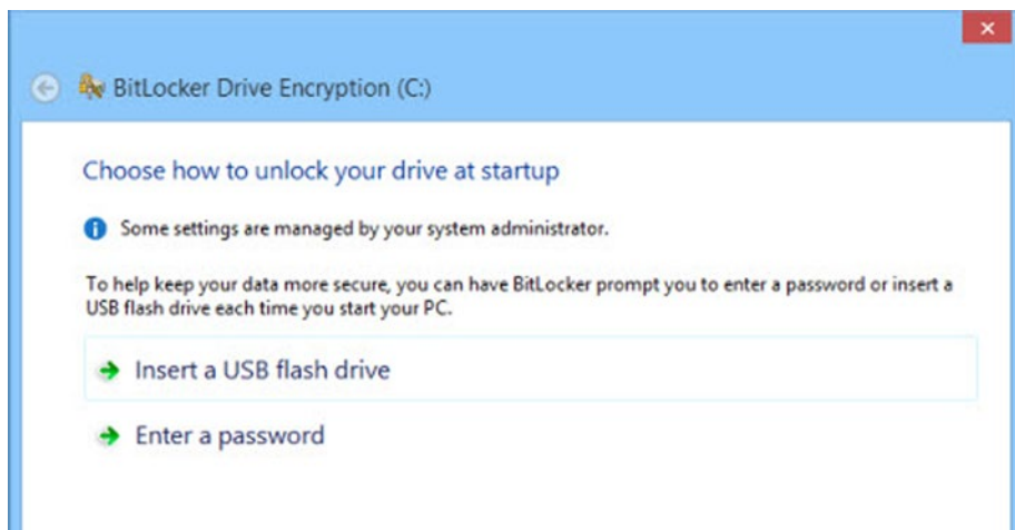
Figure 12-8. You can unlock your PC at startup with either a USB flash drive or a password
