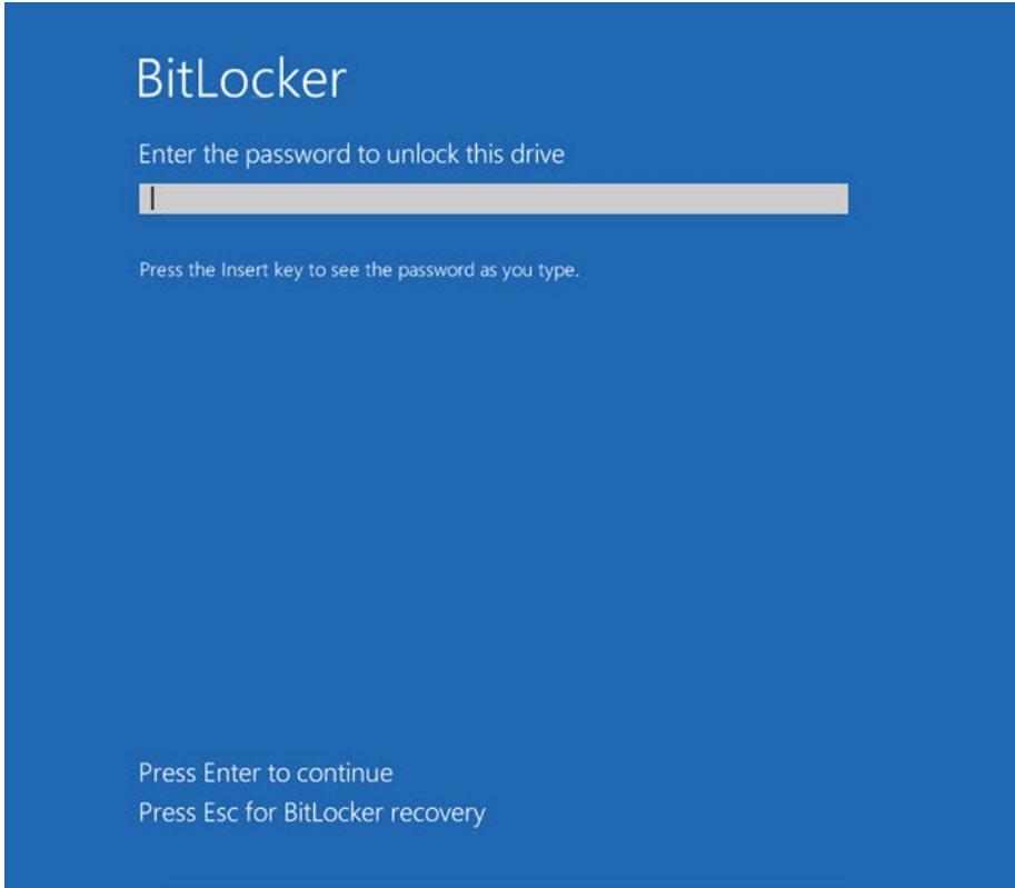
Figure 12-13. Enter your unlock password (or USB key) to make sure that it works. (Going forward, you'll also need to do this each time you start your BitLocker-encrypted PC.)
