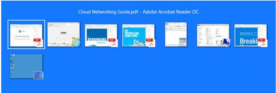
Figure 9-7. Use ALT+TAB to view and switch between all open files and apps (Windows 8.1)
