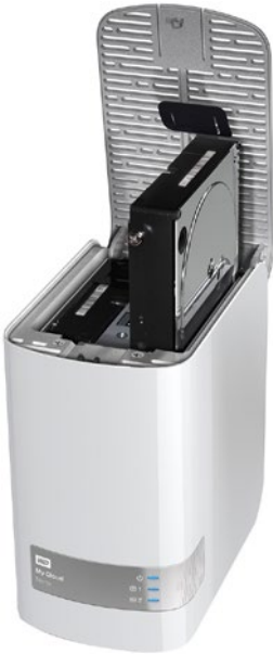
Figure 10-7. NAS devices such as the WD My Cloud mirror use multiple internal hard disks to store, share, and protect your data
