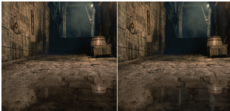
Figure 1.5. SSR only (left) and SSR blended with IBR (right). [Image courtesy Square Enix Ltd.]
