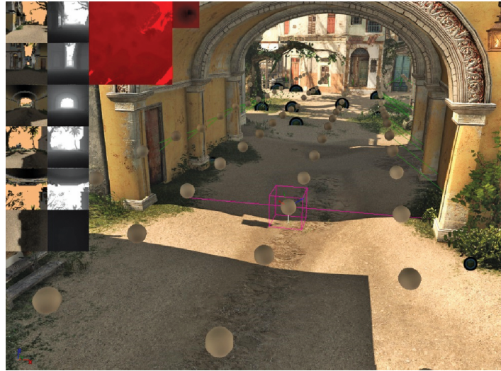
Figure 2.8. Implemented GI baking debugging tools. Top left inset, from left to right: the six faces of the normalized cube map for the current time of day, the associated depth for those faces, the current sector shadowmap, and the runtime heightmap texture (see Section 2.4.3).
