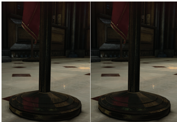
Figure 1.7. Reflection without bump (left) and with bump as a postprocess (right). [Image courtesy Square Enix Ltd.]
