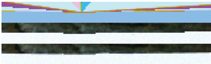
Figure 3.5. Top to bottom: a visualization of analytical distance to edge, rasterized edge, analytically antialiased edge, an edge using 5-bit gradients, and an edge showing minor artifacts when multiple triangles intersect one pixel.
