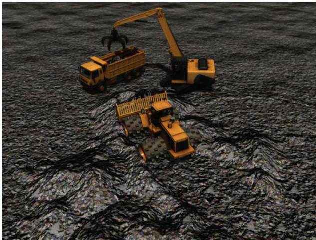
Figure 1.1. Dynamic terrain simulation in action with max (0.1 m) resolution rendered with 81,000 tris in two batches.
