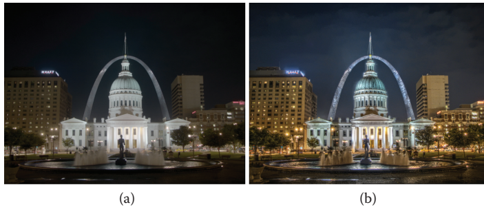
Figure 4.2. HDR images obtained using (a) global and (b) local tone-mapping operators. [Image from [McCoy 08].]
