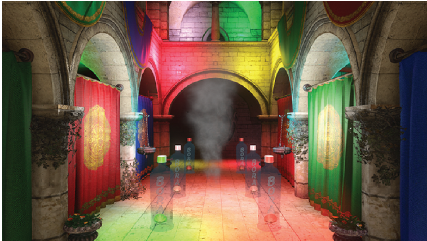
Figure 1.1. Smoke effect and translucent water bottles don't receive any scene lighting in a traditional deferred lighting engine.
