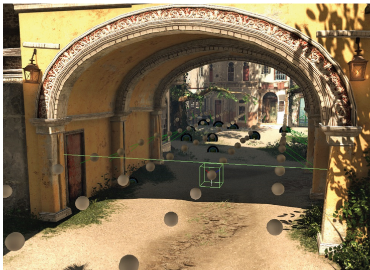
Figure 2.5. Example probe placement—regular grid.
