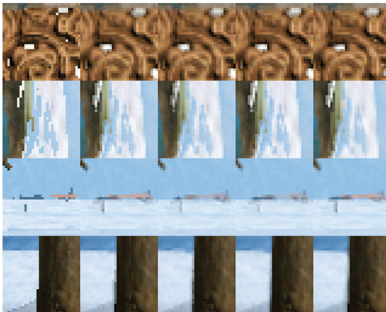
Figure 3.25. Comparison of different HRAA setups showing different scenarios based on actual game content. From left to right: centroid sampling (no antialiasing), temporal FLIPQUAD (TFQ), AEAA + TFQ, CRAA + TFQ, and SMAA + TFQ.
