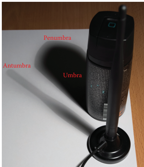
Figure 1.1. A real-life umbra, penumbra, and antumbra. The objects are lit by a desk spot lamp.
