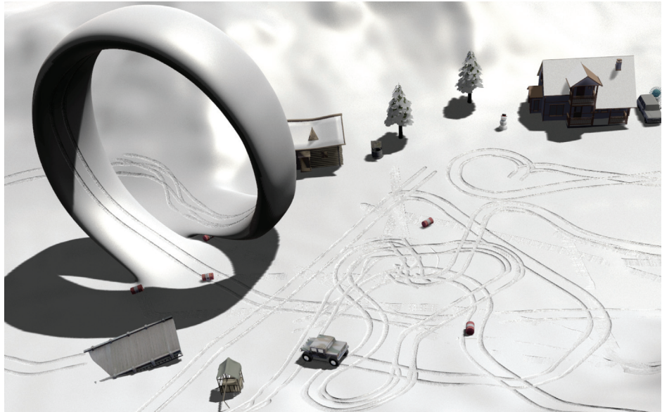
Figure 3.1. Our method allows computation and application of fine-scale surface deformations on object collisions in real time. In this example, tracks of the car and barrels are generated on the fly as the user controls the car.
