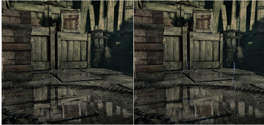
Figure 1.4. Non-glossy reflection rendering (left) and CHGR (right). [Image courtesy Square Enix Ltd.]
