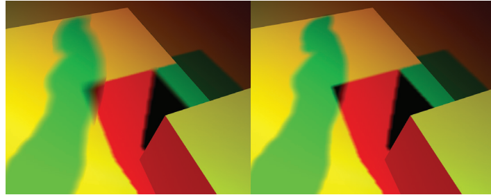
Figure 1.3. Not handling overlapping shadows properly by using layers can lead to artifacts (left), and correct overlapping shadows (right).
