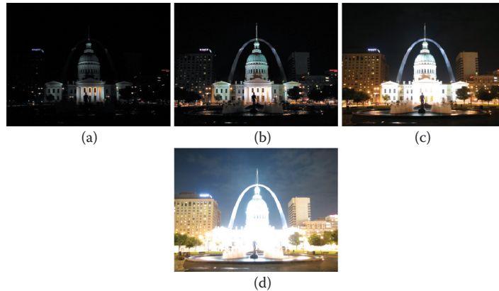
Figure 4.1. Images taken with different exposures: (a) -4 stops, (b) -2 stops, (c) +2 stops, and (d) +4 stops. [Image from [McCoy 08].]
