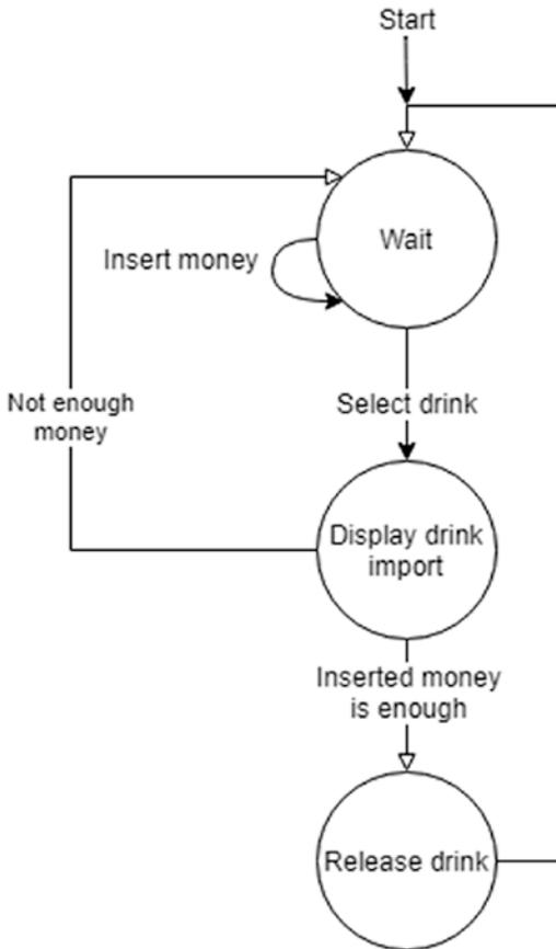
**Figure 4-1.** FSM scheme of a vending machine
