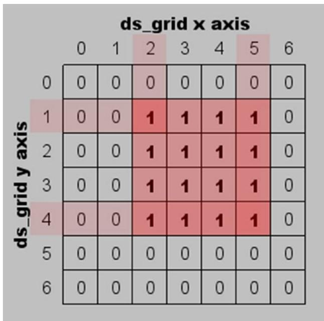
**Figure 12-2.** The pink square is a grid region inside a DS Grid. This specific region starts at (1,2) and ends at (4,5).
