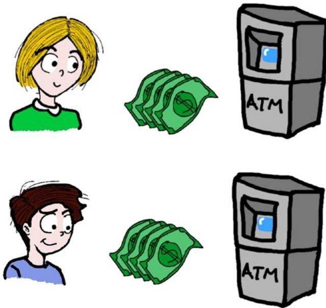
**Figure 12-4.** Alice and Bob both receive \$40 from the ATM, even if they have just \$50 in their shared account. This is because the race condition wasn't addressed by the ATM programmer.
