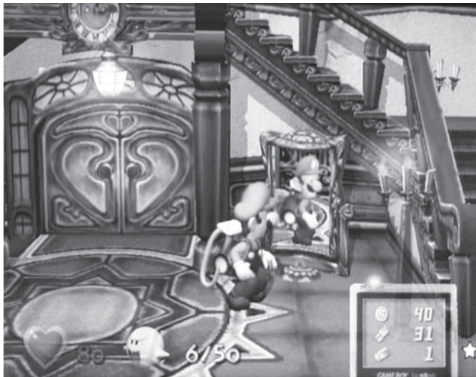
Figure 10.54. Mirror reflections in Luigi's Mansion implemented by rendering the scene to a texture that is subsequently applied to the mirror's surface.
