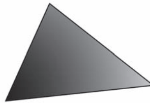
Figure 10.11. A Gouraud-shaded triangle with different shades of gray at the vertices.
