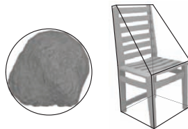
Figure 12.1 Simple geometric shapes are often used to approximate the collision volumes of the objects in a game.
