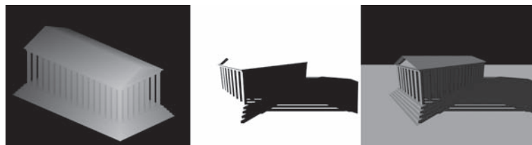
Figure 10.52. The far left image is a shadow map—the contents of the z-buffer as rendered from the point of view of a particular light source. The pixels of the center image are black where the light-space depth test failed (fragment in shadow) and white where it succeeded (fragment not in shadow). The far right image shows the final scene rendered with shadows.
