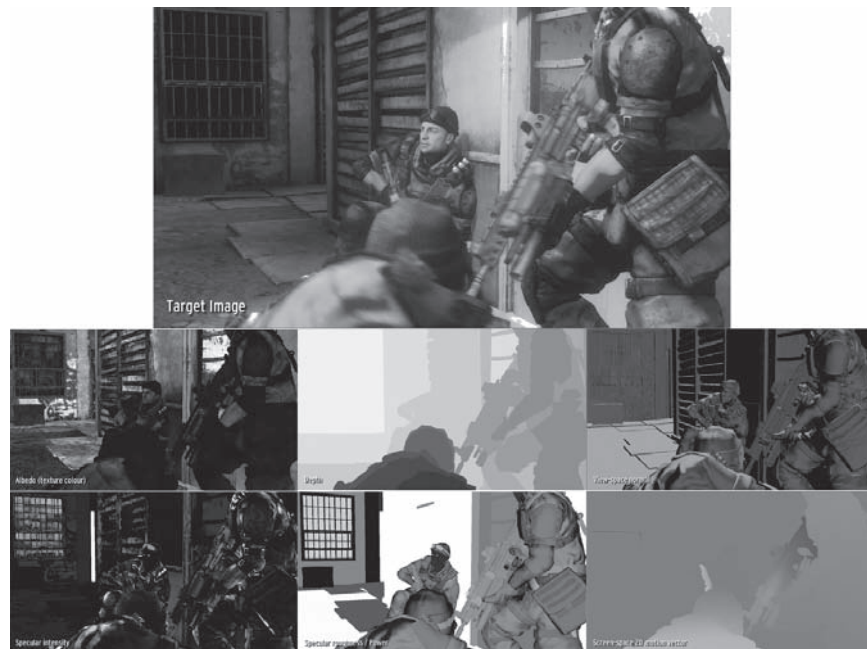
Figure 10.57. Screenshots from Killzone 2 , showing some of the typical components of the G-buffer used in deferred rendering. The upper image shows the final rendered image. Below it, clockwise from the upper left, are the albedo (diffuse) color, depth, view-space normal, screen space 2D motion vector (for motion blurring), specular power, and specular intensity.
