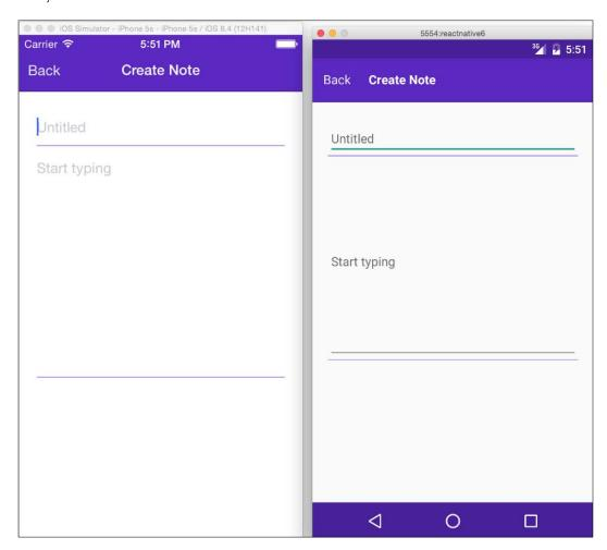
This doesn't look right on Android yet. The TextInputs on Android have a default underline and they center the text vertically on multiline inputs. There are two Android only attributes that can be added to match the look of the iOS application. On each TextInput set the underlineColorAndroid as transparent and textAlignVertical on the body as TextInput:
