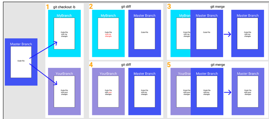
FIGURE 1-1: Example workflow for Git branches.
