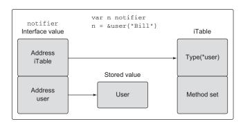
Figure 5.2 A simple view of an interface value after concrete type pointer assignment
