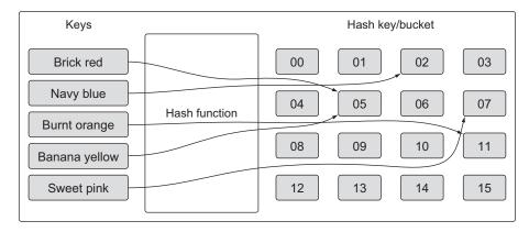
Figure 4.25 Simple view of how hash functions work
