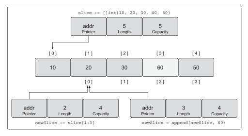
Figure 4.14 The underlying array after the append operation
