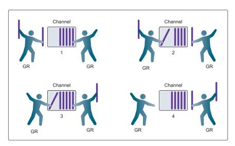
Figure 6.7 Synchronization between goroutines using a buffered channel
