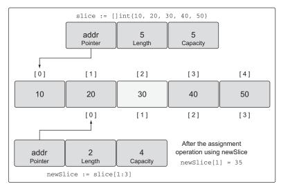
Figure 4.13 The underlying array after the assignment operation
