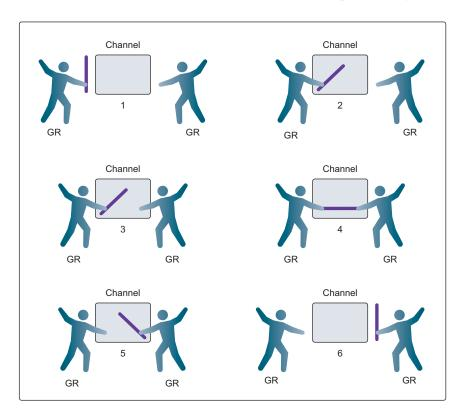
Figure 6.6 Synchronization between goroutines using an unbuffered channel
