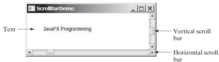
FIGURE 16.23 The scroll bars move the message on a pane horizontally and vertically.
