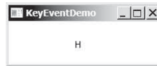
FIGURE 15.13 The program responds to key events by displaying a character and moving it up, down, left, or right.
