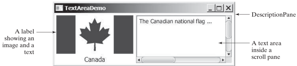
FIGURE 16.14 The program displays an image in a label, a title in a label, and text in the text area.
