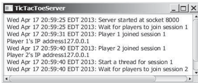
FIGURE 31.15 TicTacToeServer accepts connection requests and creates sessions to serve pairs of players.
