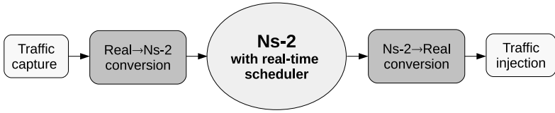
Figure 6.1. Emulation architecture of Ns-2.
