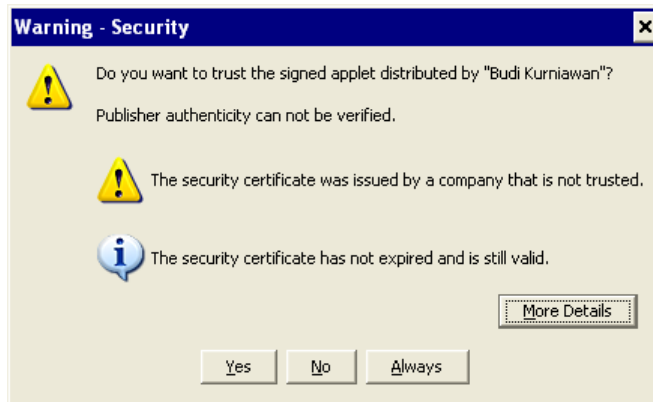
Figure 25.6: The security warning asking the user whether to grant permissions to an applet
