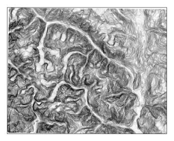
The slope shows the gradual decline in elevation from the high points to low points in all the directions of the dataset. Slope is an especially useful input for many types of hydrology models.
