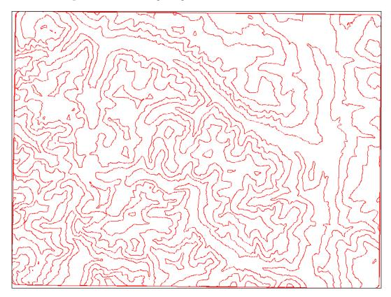
If we bring our shaded relief ASCIIGRID and the shapefile into a GIS, such as QGIS, we can create a simple topographic map as follows. You can use the elevation (that is *ELEV*) dbf field that you specified in the script to label the contour lines with the elevation:
