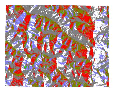
The aspect shows the maximum rate of downslope change from one cell to its neighbors. If you compare the aspect image to the shaded relief image, you can see that the red and gray values of the aspect image correspond to shadows in the shaded relief. So, the slope is primarily responsible for turning the DEM into a terrain relief while the aspect is responsible for the shading.
