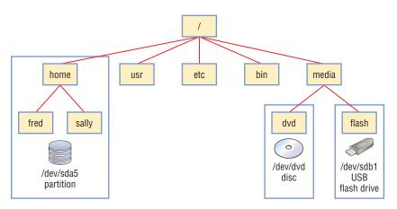
FIGURE 7.2 In Linux, all files are referenced relative to a single root (/) directory.
