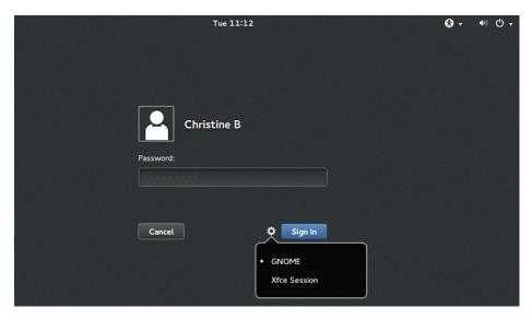
**FIGURE 4.1** GUI login managers usually provide a selection of desktop environments from which you can choose.
