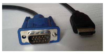
**FIGURE 5.4** VGA connectors (left) were common in years past and are still available today; HDMI connectors (right) are common on newer monitors and video cards.
