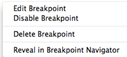
Figure 11-8: The list of operations you can use to modify the behavior of a breakpoint.
