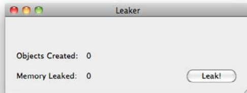
Figure 12-14: The Leaker main window. Each click of the button creates new objects and loses track of them all.
