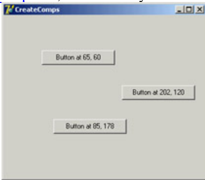
Figure 2.1: The output of the CreateComps example, which creates Button components at run time
