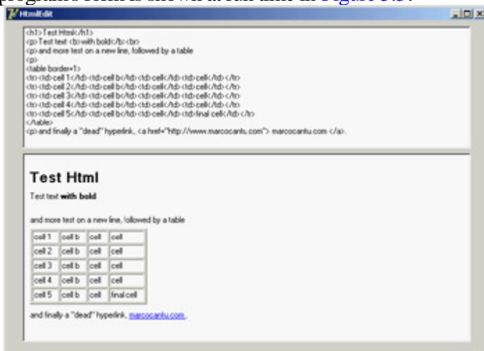
Figure 5.3: The HtmlEdit example at run time: When you add new HTML text to the memo, you get an immediate preview.
