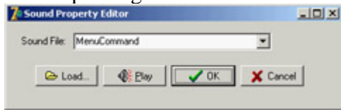
Figure 9.13: The Sound Property Editor's form displays a list of available sounds and lets you load a file and hear the selected sound.
