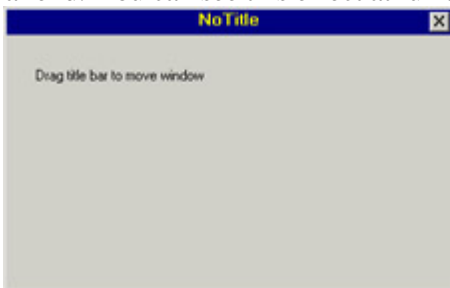
Figure 7.4: The NoTitle example has no real caption but a fake one made with a label.
