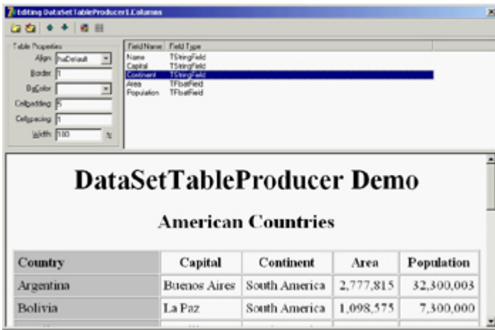
Figure 19.9: The editor of the DataSetTable-Producer component's Columns property provides you with a preview of the final HTML table (if the data-base table is active).
