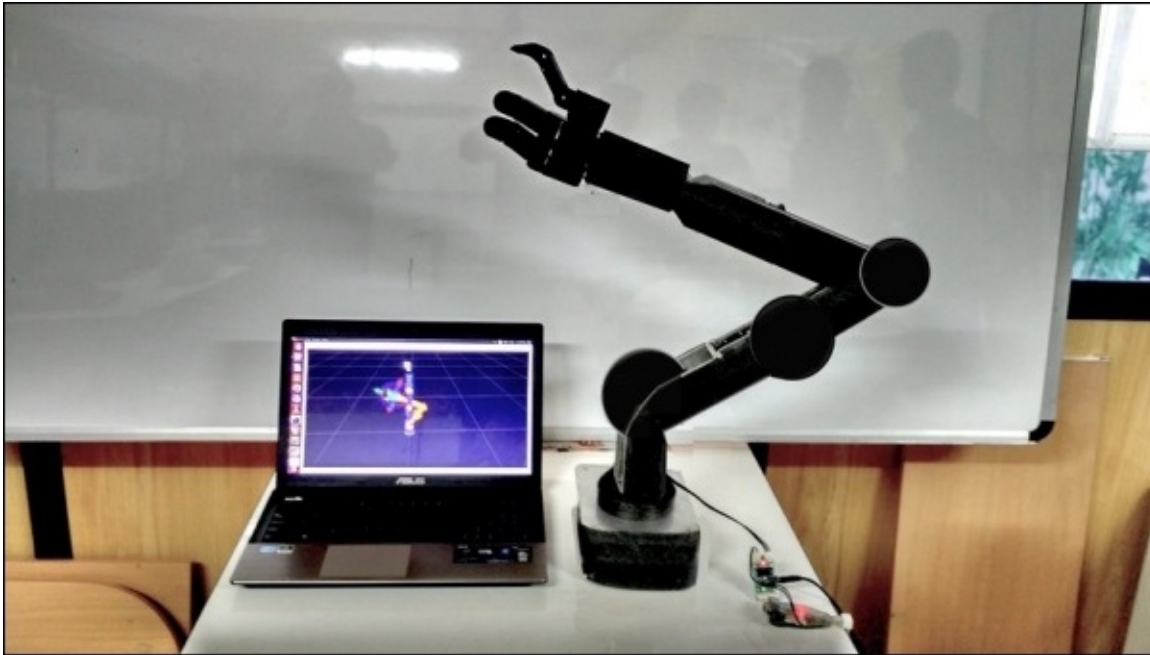
Figure 16 : COOL-Arm-5000 prototype with MoveIt! visualization
