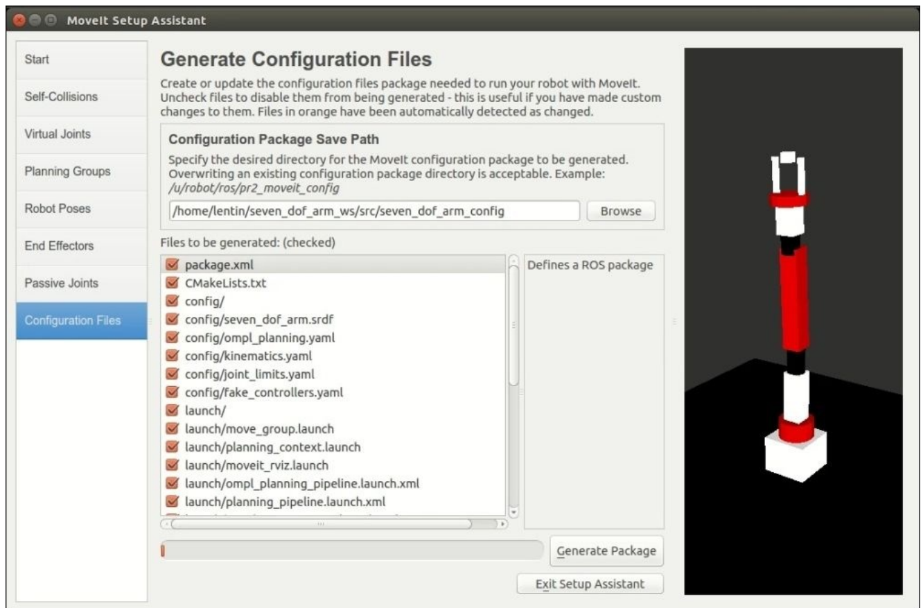
Figure 10 : Generating the MoveIt! configuration package
