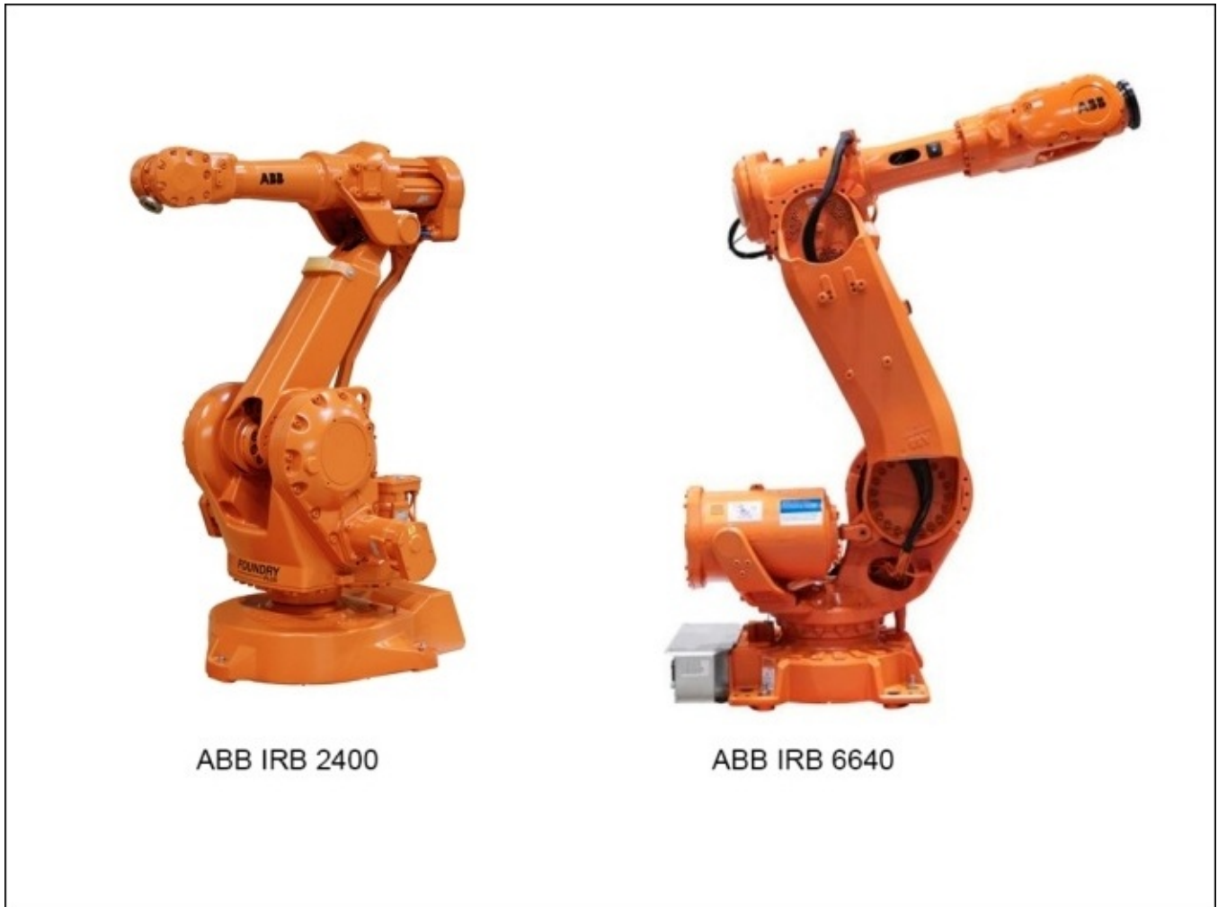
Figure 11: ABB IRB 2400 and IRB 6640
