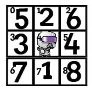
The big bold numbers represent the order in which tile collisions are handled, bottom first, top second, left-hand side third, and right-hand side fourth, then the corners. The smaller numbers represent the order in which those tiles are stored in the tileIndex variable.
