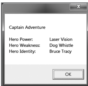
Figure 11.8 The SuperHero object's DisplayIdentity() method displays the value of all properties assigned to an instance of an object. © 2014 Cengage Learning.
