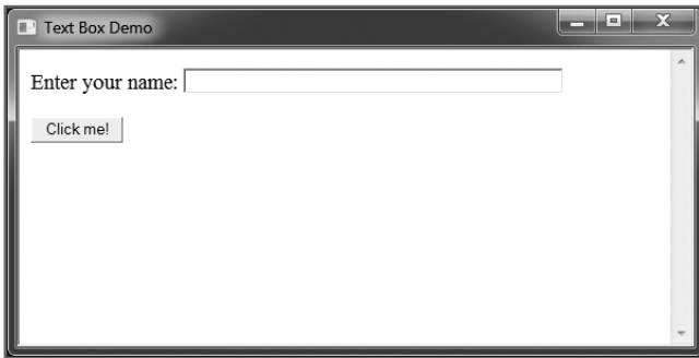
Figure 14.9 An HTA whose GUI includes a text control and a button control. © 2014 Cengage Learning.
