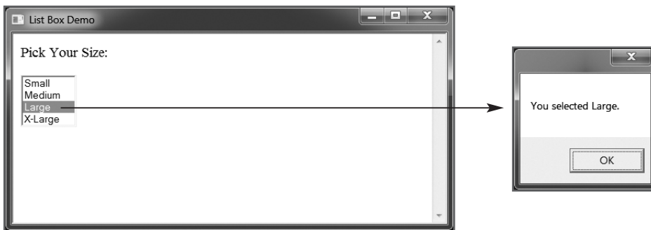
Figure 14.15 A list box control configured to trigger the execution of a script whenever an item is selected.
