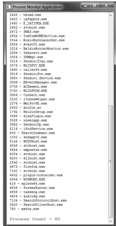
Figure 14.19 This HTA auto-refreshes every second to provide up to date process data collected via WMI.
