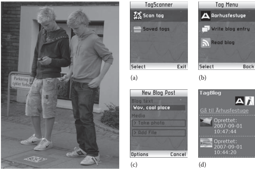
Figure 7.8 The mobile phone blogging user interface. (a) Scanning a TAG to identify the context. (b) choosing the action. (c) Creating a multimedia blog post. (d) Viewing the blog that is anchored on the TAG.
