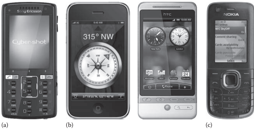
Figure 7.4 Off-the-shelf mobile devices with sensor capabilities. (a) Camera phone. (b) Sensor enabled smart phones. (c) RFID enabled mobile phone.
