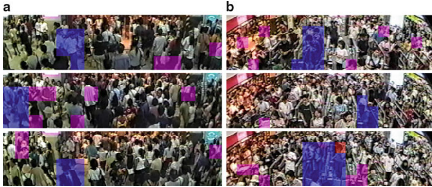
Fig. 10.4 (Color online) Our crowd flow model enables the detection of local unusual activities such as pedestrians moving against the crowd by examining the deviation of observed local motion patterns from the learned crowd flow model. Blue : true positive, Magenta : false positive, and Red : false negative
