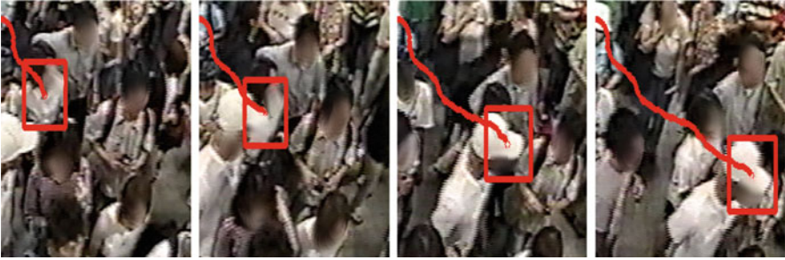
Fig. 10.14 Example of a tracking failure due to severe (near full) occlusion
