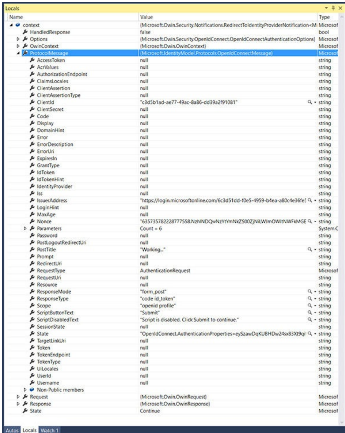
Figure 7-15 The content of the context parameter on a typical RedirectToIdentityProvider notification execution.
