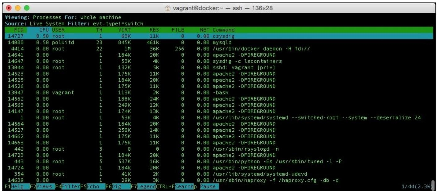
The screenshot shows the Csysdig interface in a terminal window. The title bar indicates the user is 'vagrant@docker' in an SSH session. The main display shows a table of processes with columns for PID, CPU, USER, TH, VIRT, RES, FILE, NET, and Command. The 'csysdig' process is highlighted in blue. At the bottom, there is a keyboard shortcut menu and a status bar showing '1/44(2.3%)'.
