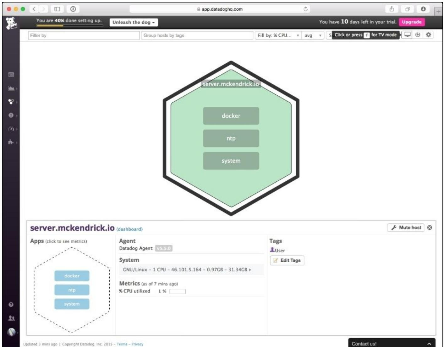
The screenshot shows the Datadog web interface for a host named `server.mckendrick.io`. The main area displays a large green hexagon representing the host, with three smaller green boxes inside labeled `docker`, `ntp`, and `system`. Below this, the dashboard provides detailed information:
