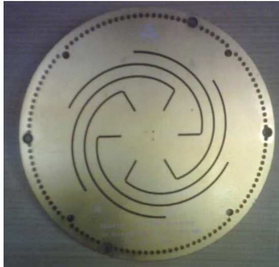
Figure 3.1: GNSS fixed radiation pattern antenna element.
