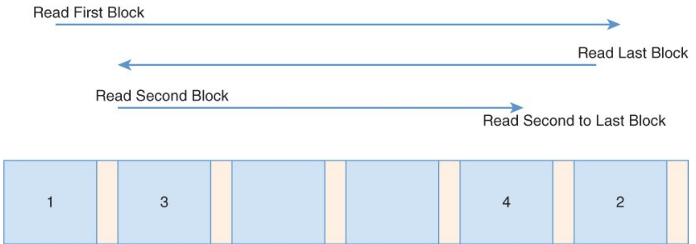
Figure 1.3 Random access to blocks on tape can take more time than sequential access because there can be more tape movement relative to the amount of data read.
