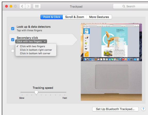
Figure 5-15: The Trackpad System Preference pane offers controls for one-finger and multi-finger gestures.
