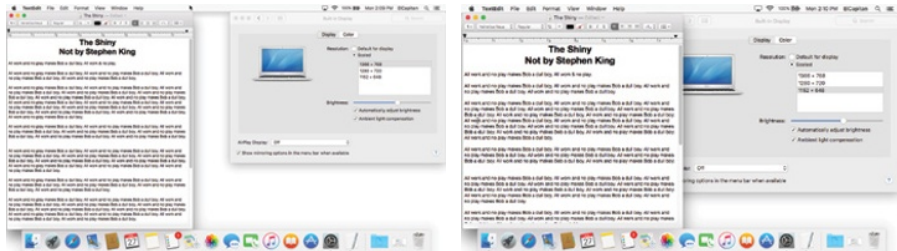
Figure 21-2: My MacBook Air at its highest resolution, 1366 x 768 (left), and its lowest, 1152 x 648 (right).
