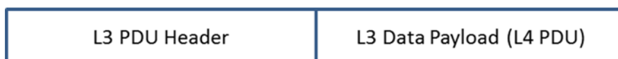
Figure 5-2. The general form of an IP protocol data unit or IP datagram
