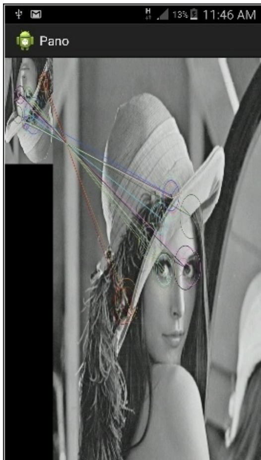
Native matching using ORB for feature detection and description
