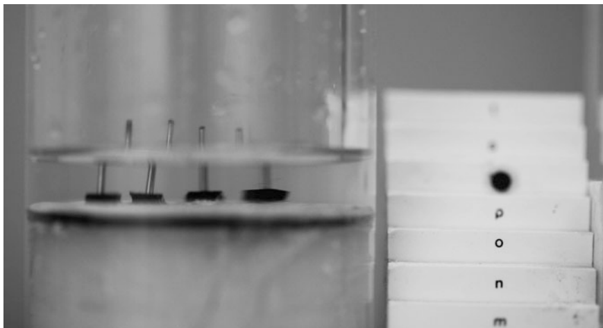
Fig. 15 Frontal image showing focus on the second deeper metallic pin. A focus stair is positioned besides the tube
