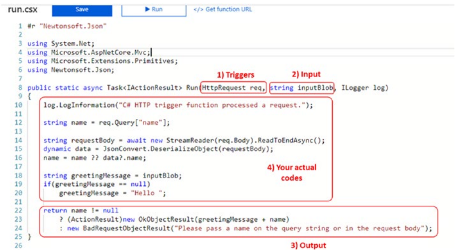
Figure 2-2. An example of an actual function (run.csx)
