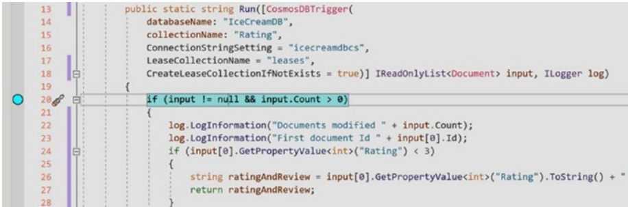
Figure 4-14. Toggling the breakpoint in Azure Functions code in Visual Studio
