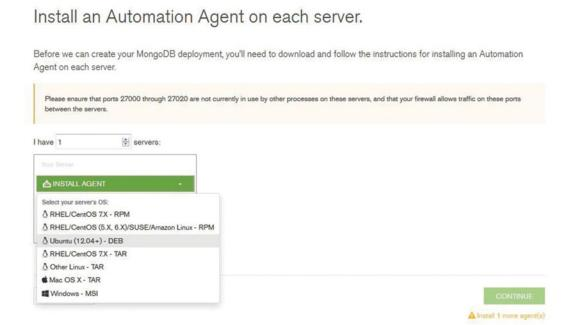
Figure 5-5. Installing an automation agent
