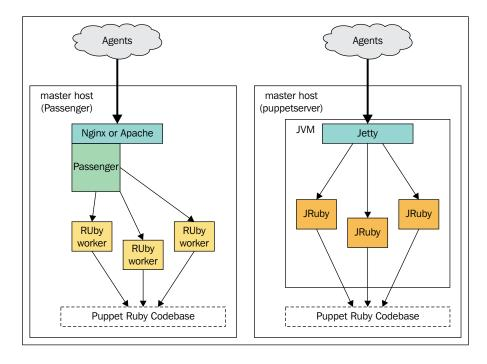
With puppetserver, both the web service and the Ruby runtimes share a single JVM. This allows a better overall performance, and is easier to set up. All new setups should therefore, prefer puppetserver over Passenger.
