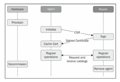
The very first step – generating a key and a certificate signing request – is always performed implicitly and automatically at the start of an agent run if no local SSL data exists yet. Puppet creates the required data if no appropriate files are found. There will be a short description on how to trigger this behavior manually later in this section.
