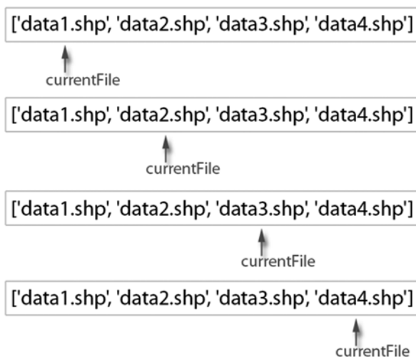
Figure 10.1 Python automatically updates the variable, currentFile in Example 10.3, to each item in the list.
