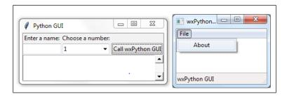
In the previous code, we inherited from wx. Frame. In the following code, we inherit from wx. Panel and we pass in wx. Frame to the init () method of our class.
