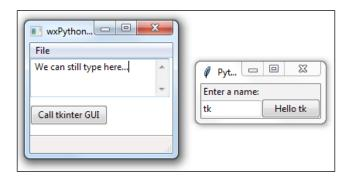
After starting the tkinter event loop, the wxPython GUI is still responsive because we can type into the TextCtrl widget while the tkinter GUI is up and running.
