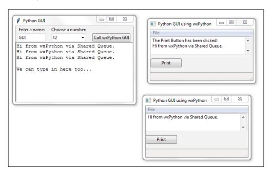
The tkinter GUI is shown on the left-hand side of the preceding screenshot and, by clicking the **Call wxPython GUI** button, we invoke an instance of the wxPython GUI. We can create several instances by clicking the button several times.
