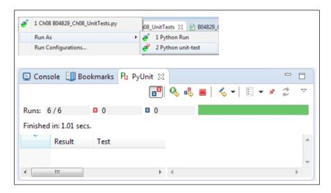
The unit testing result bar is green, which means that all our unit tests have passed. The preceding screenshot also shows that the GUI test runner is much slower than the textual test runner: 1.01 seconds compared to 0.466 seconds in Eclipse.
