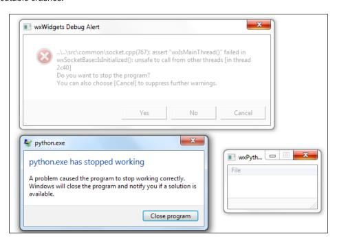
In order to avoid this, instead of trying to run the entire wxPython application in a thread, we can change the code to make only the wxPython app.MainLoop run in a thread.
