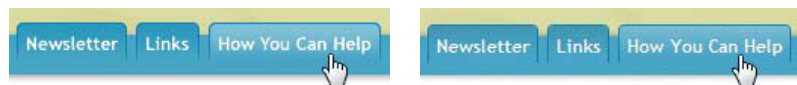
FIGURE 1.6 The image tabs (left) look almost identical to the tabs made with CSS3 (right).
