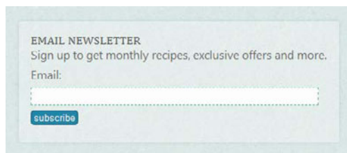
FIGURE 7.22 In browsers that don't support flexible box layout (like Opera 10.6, shown here), each element of the form is on its own line instead of sitting side by side.
