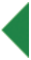
FIGURE 2.7 Making all but one of the borders transparent creates the appearance of a single triangle.
