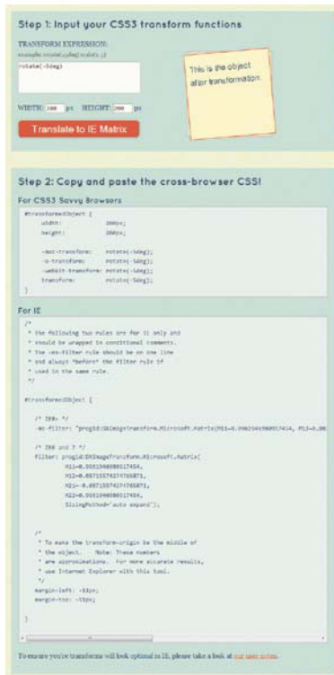
FIGURE 2.26 The Transforms Translator web site generates IE Matrix filter values that are equivalent to the CSS3 2D transforms you feed it.
