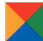
FIGURE 2.6 When a box has no width or height, each border creates the appearance of a triangle.
