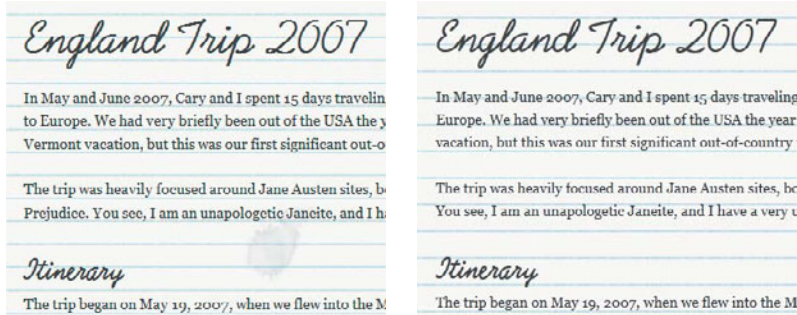
FIGURE 3.30 Different platforms and browsers, such as Firefox 3.6 (left) and IE 9 (right), display the anti-aliasing of the headings differently.
