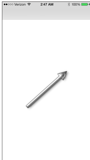
Figure 14-1 A little math recovers the “up” direction by performing an arctan function using the x and y force vectors. In this example, the arrow always points up, no matter how the user reorients the device.
