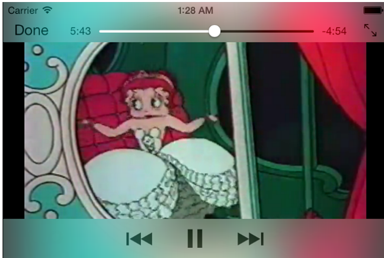
Figure 8-3 The Media Player framework simplifies adding video playback to your applications. This class allows off-device streaming video as well as fixed-size local assets. Supported video standards include H.264 Baseline Profile Level 3.0 video (up to 640×480 at 30fps) and MPEG-4 Part 2 video (Simple Profile). Most files with .mov, .mp4, .mpv, and .3gp extensions can be played. Audio support includes AAC-LC audio (up to 48KHz) and MP3 (MPEG-1 Audio Layer 3, up to 48KHz) stereo.
