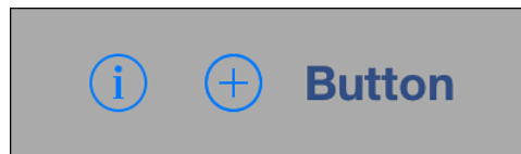
Figure 2-2 iOS SDK offers five typed buttons with three visually distinct interfaces. You can access them in IB or add them to your applications directly with code. The first symbol here represents three buttons: Detail Disclosure, Info Light, and Info Dark. The other two buttons are the Contact Add button and the System button.
