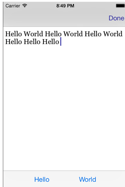
Figure 6-6 The custom keyboard attached as this text view’s input view allows users to enter Hello and World—and that’s all.
