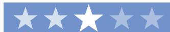
Figure 2-6 Recipe 2-6 creates a custom star slider control that animates each star upon selection. A simple animation block causes the star to zoom out and back as the control's value updates.
