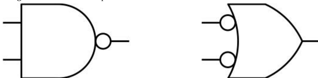
Figure 2-28: Redrawing a NAND gate using De Morgan’s law
