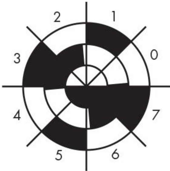
Figure 6-13: Binary rotary encoder alignment error
