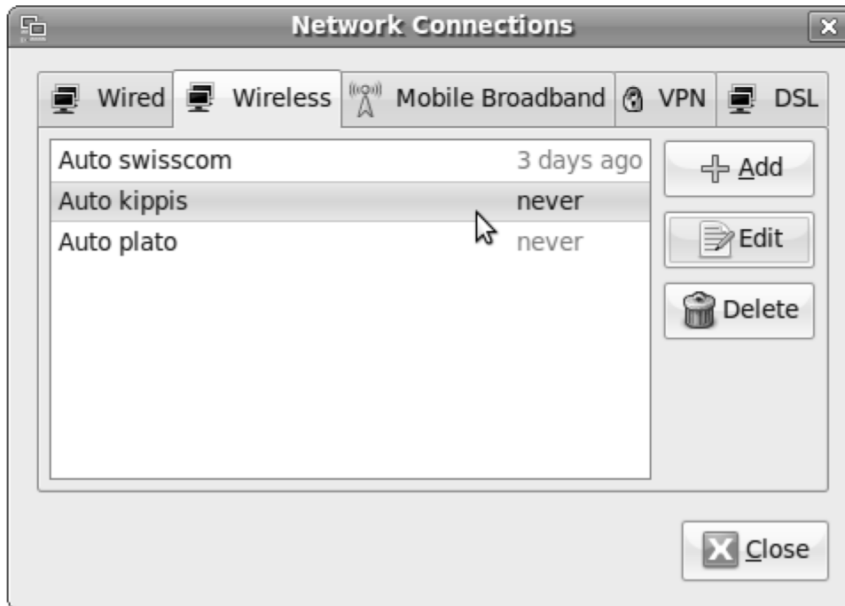
Figure 3-13. On the Wireless tab, you have access to all wireless networks you've ever accessed.
