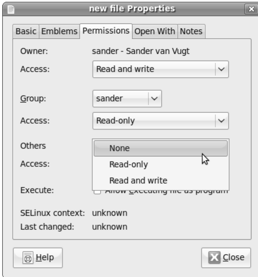
Figure 2-17. If you want to be sure you're the only one who can access a file, set the permissions for others to None.
