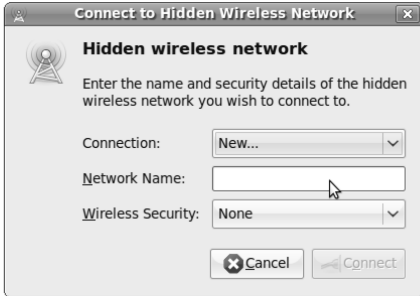
Figure 3-11. Enter the network name and security option to configure access to a hidden wireless network.
