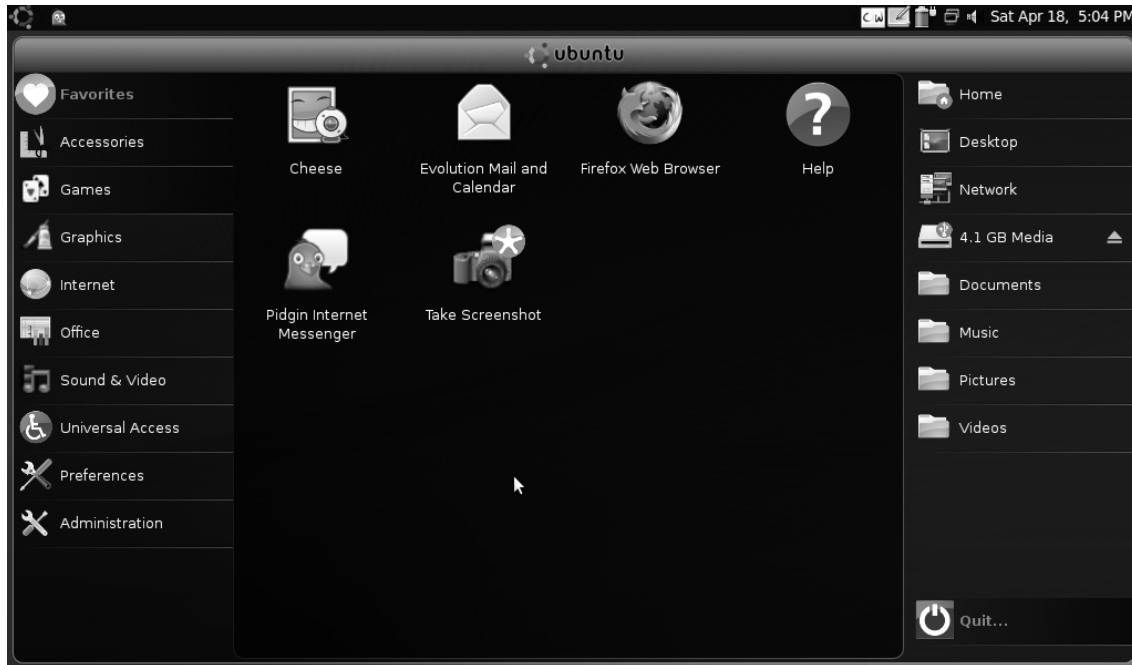
Figure 2-8. When you connect removable storage to your computer, it appears automatically in the Places section.
