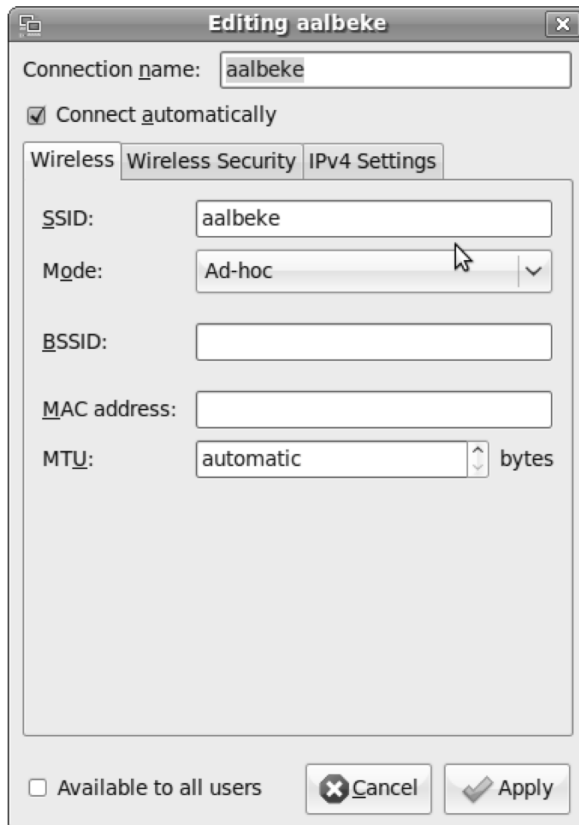
Figure 3-25. To make a connection with a wireless network, be sure you have an SSID and Infrastructure connection mode.
