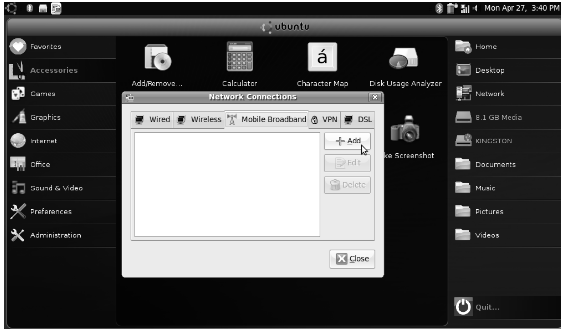
Figure 3-6. You can create the 3G network connection using the Mobile Broadband tab.
