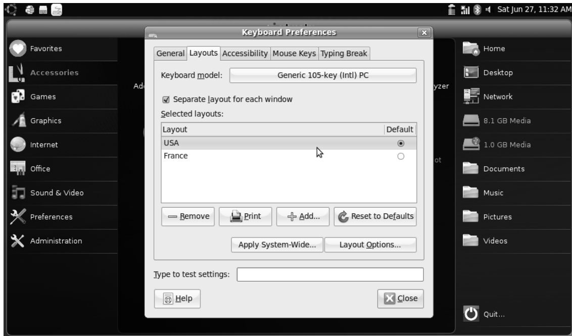
Figure 7-2. If your default keyboard layout doesn't fit your needs, add a new layout and make it the default setting.
