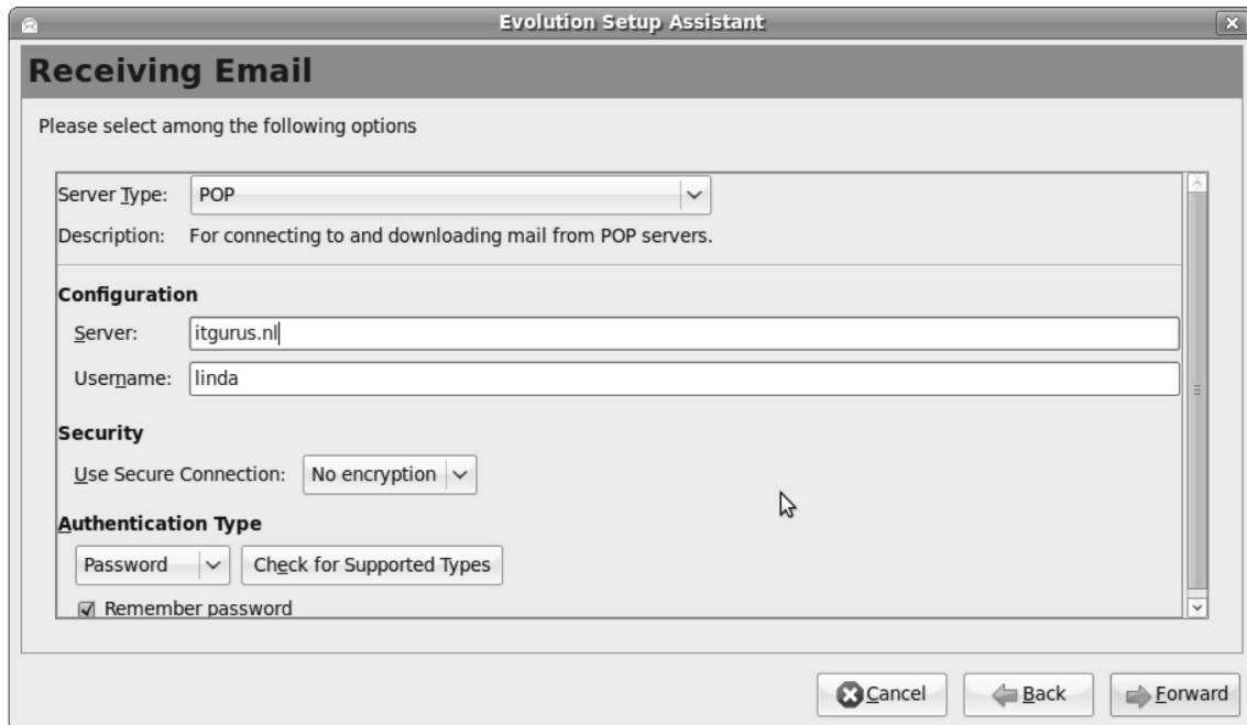
Figure 4-21. You need at least the name of the server and the name of the user account on that mail server.
